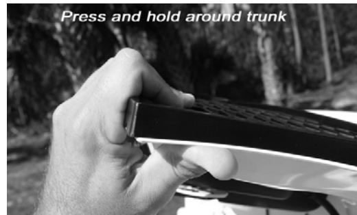
Fig. 4 – Working your way around trunk panel, grab and hold tightly for at least 30 seconds in each area
